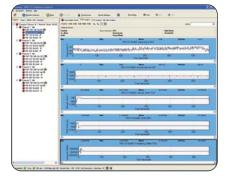
PCR graphs are available in real time and deferred time. Time stamping data ensure that these can be captured and viewed on stream recordings. This timestamp is compatible with recordings from other Tektronix equipment, including the MTM400 Transport Stream monitor. Selectable MGF filters provide maximum flexibility and compatibility in these important PCR measurements.
